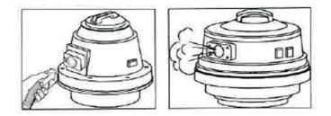
Push hose into blower port placed on the vacuum head. Turn the switch on.
